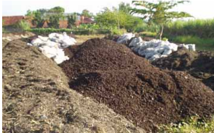
Figure 1. Filter cake (above) and ash of bagasse (left, below) are the main waste from sugar cane factory
